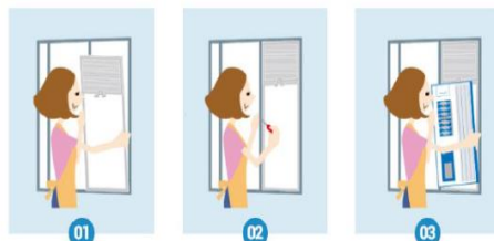
01 Tighten the bolts to secure the installation kit. 02 Mount the installation kit on the window. 03 Install the air conditioner in the installation kit
